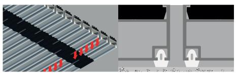
The main feature that makes EXPERT superior lies in its innovative connection system between profiles which uses a polyamide hinge, this allows ALL THE DIRT gathered between the profiles to remain deposited at the bottom of the matwell, it will suffice to simply roll up the mat and remove the captured dirt accumulated in the matwell in which it is housed
