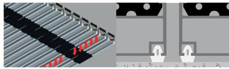
The main feature that makes EXPERT superior lies in its innovative connection system between profiles which uses a polyamide hinge, this allows ALL THE DIRT gathered between the profiles to remain deposited at the bottom of the matwell, it will suffice to simply roll up the mat and remove the captured dirt accumulated in the matwell in which it is housed
