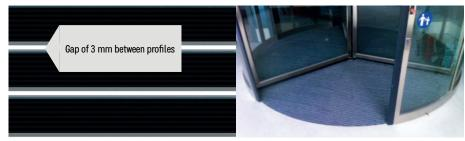
In accordance with EN 16005 for those entrance mats fitted under a revolving door gap between profiles shouldn't exceed 4 mm Gap between HERCULES profiles is 3 mm, which makes HERCULES the right choice for those cases in need to meet EN standards when it comes to automatic revolving doors
