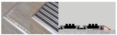
Aluminium ramp profile for creating a matwell over the floor, valid exclusively for 10 mm high doormats, useful for those cases where there is no matwell in which to accommodate the doormat
