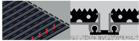
Its main feature is that aluminium profiles are joined together by a high strength PVC joint allowing the mat to be rolled up in order to make its handling easier or to perform periodic removal of the dirt
